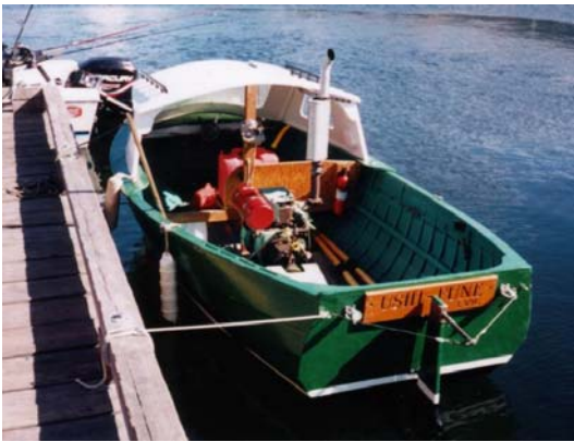
The 1951, 4-horsepower Wisconsin cast-iron one-lunger came complete with the original manual.
